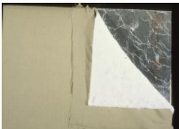
spatula. Because polyethylene melts at a fairly low temperature, about 170°C (335°F), domestic irons set to the "permanent press" setting are usually adequate to fuse the polyethylene to the surface beneath. However, the heat must be applied evenly to the entire surface to ensure proper melting and good adhesion. Any holes or tears can easily be repaired by ironing a patch of the same aluminum barrier foil over the damaged area.
